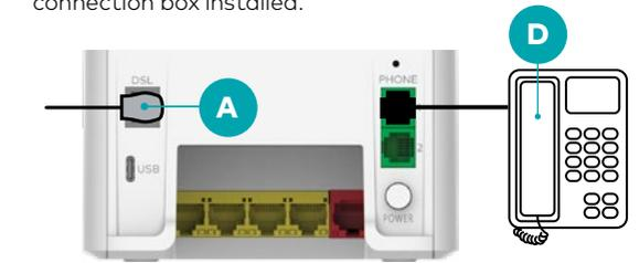
**A.** Plug one end of the telephone cable (grey connectors) into the grey port on your modem, labelled DSL.
