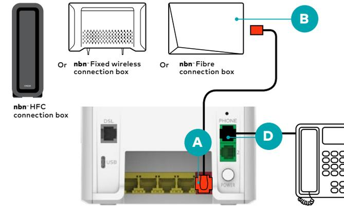
**A.** Take the ethernet cable (red connectors) and plug one end into the red port on your modem labelled WAN.
